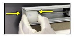
CAUTION: REMOVED SPRINGS WILL BE PRELOADED! Failure to securely hold the spring assembly together during removal could cause separation of the spring housings allowing the spring to quickly unwind, expanding outside the housing, and potentially LEAD TO INJURY.
