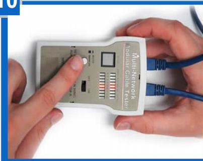
Repeat Steps for other end of cable. Use a cable tester to ensure proper installation and wiring of plugs.
