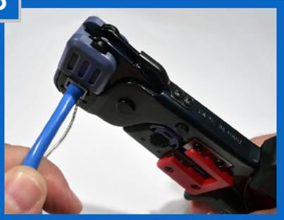
Crimp the plug using the crimp tool. Place the plug into the crimp tool and squeeze handles tightly. The copper splicing tabs on the plug will pierce into each of the eight conductors. The locking tab will cinch onto the outer jacket of the cable.
