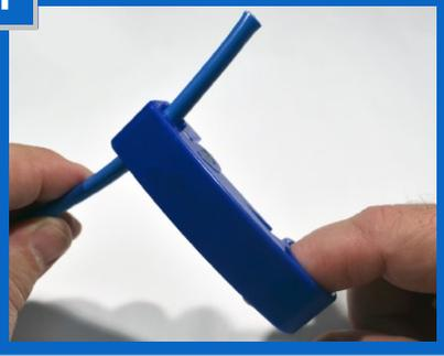
Cut cable to the desired length. Remove the outer jacket of the cable using stripping tool. Place the tool approximately 1.25" from the end of the cable. Rotate the tool at least twice around the cable, both clockwise and counter-clockwise. That will score the jacket allowing you to remove it without damaging the conductors inside.
