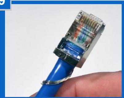
Remove the plug from tool. Check the conductor sequence and ensure outer jacket is inside the plug and secured by the locking tab. For shielded cable applications - trim the excess drain wire just below entry into plug.
