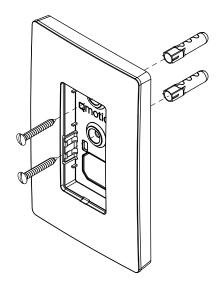
**IMPORTANT:** Make sure to install the Locking Station in the correct orientation. The back of the Locking Station has an indication in the upper right corner.
